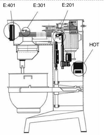
**E:201** The servo motor block actuator (B) did not contact the minimum speed microswitch (A) after
